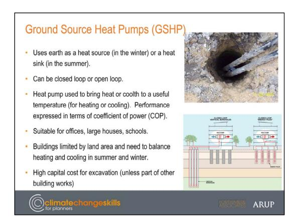
CoP = Coefficient of Power or Coefficient of Performance. This is the ratio between the heat generated and the electricity consumed by the heat pump.
