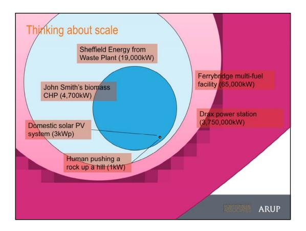
The area of each of these circles equates to the rated or peak power output of selected energy generation facilities. It highlights the effect of scale and helps to keep a perspective on the ability of small-scale renewable energy to replace large-scale centralised power stations.
