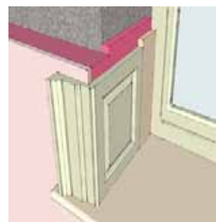
Internal wall insulation options would need careful detailing to contain new insulant (dark pink) behind removed and replaced window reveals.
