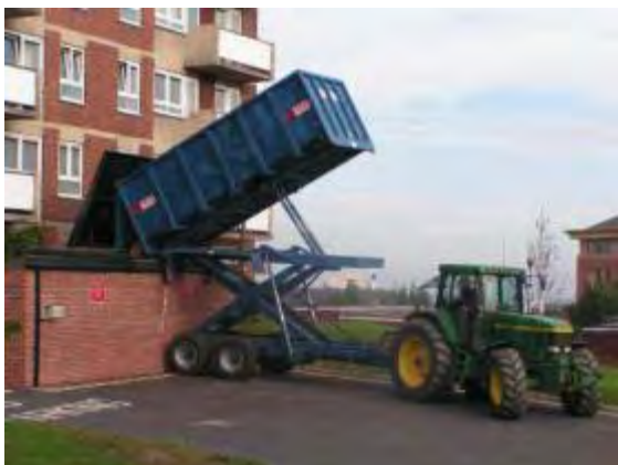
Figure 31 Delivery of biomass at Sheffield Road flats, Barnsley (Source: Case study – Sheffield Road – Barnsley MBC)
